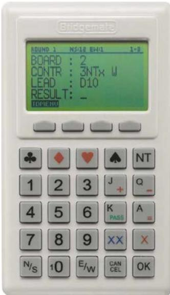
**1 to 9, 10** These keys are used to enter numbers in the Bridgemate, for example board numbers, pair numbers, contract and result. The 10 button is used to enter 0 (when entering member numbers, board numbers, etc.) and to indicate 10 as the lead card.
