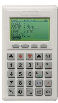
**1** to **9**, **10**; keys to enter numbers in the BridgeMate. *E.g. board numbers, pair numbers, contract, and result.* The **10** button is used to enter **0** (when entering member numbers, board numbers, etc.) and to indicate **10** (when entering lead card).
